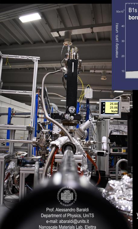
Photoelectron spectroscopy is an ideal tool to investigate the structural, electronic and chemical properties of 2D materials, to follow in-situ their growth process and to understand their thermal behaviour in a temperature range that can be finely tuned from 20 to 1000 K.
